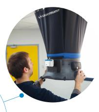
Air flow control at the inlet and outlet of a room, ventilation balancing and calculation of the air change rate. Also controls the temperature and hygrometry of the air.
