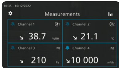
Trend indicator: up to 4 parameters displayed simultaneously
