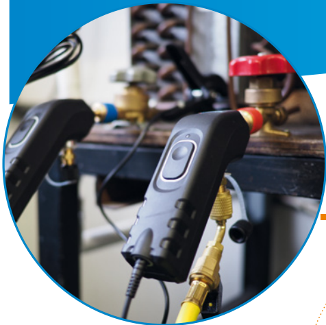
TAKE COOLING UNIT MEASUREMENTS WITH THE SI-RM3
