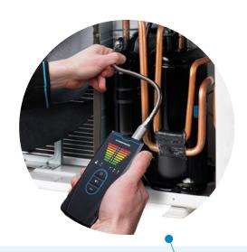
Detect most refrigerant gas leaks throughout a heat pump gas loop.
