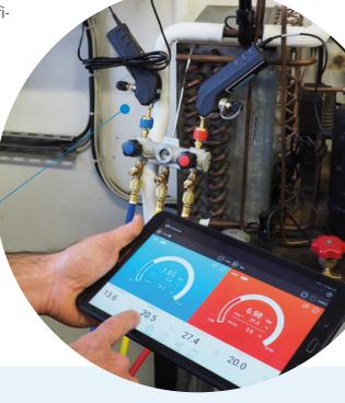
This tool allows the user to commission a heat pump, check the refrigerant circuit tightness or fill gas and check differential pressure and subcooling / superheating temperatures simultaneously.
