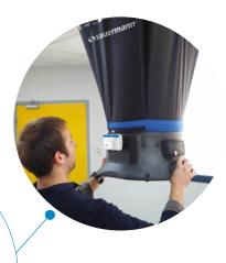
Air flow control at the inlet and outlet of a room, ventilation balancing and calculation of the air change rate. Also controls the temperature and hygrometry of the air.
