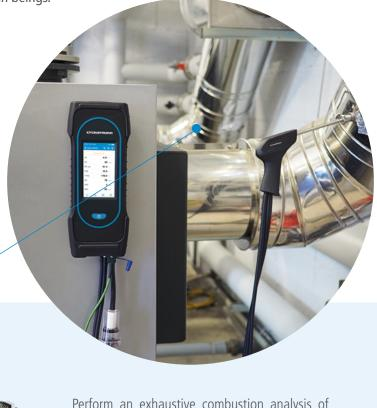
Perform an exhaustive combustion analysis of a residential or commercial boiler or furnace with an efficiency test, CO and NOx emissions measurements, calculation of CO<sub>2</sub>, CO ambient monitoring, and stack draft (pressure) and temperature measurements.
