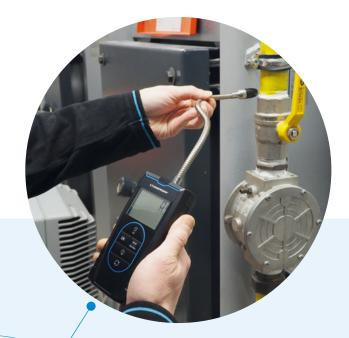
Detect any combustible gas leaks, such as natural gas, methane, propane, isobutane, and LPG, throughout a boiler's gas piping system.
