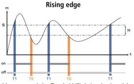
Measurement (m) > Threshold (S) during the time-delay T1  $\rightarrow$  Relay activation
