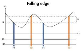
Measurement (m) < Threshold (S) during time-delay T1  $\rightarrow$  Relay activation.
