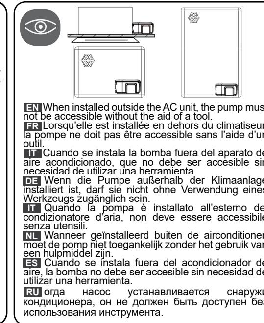
**EN** When installed outside the AC unit, the pump must not be accessible without the aid of a tool.
