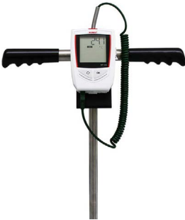
Fastening on stand with temperature data logger
