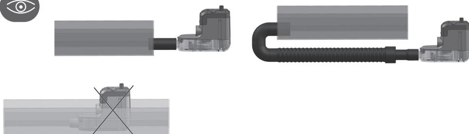
**EN** When installed outside the AC unit, the pump must not be accessible without the aid of a tool.
