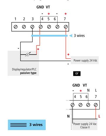
For **TM110 – PO** and **TM110 – PN** models with 4-20 mA output – **passive**:
