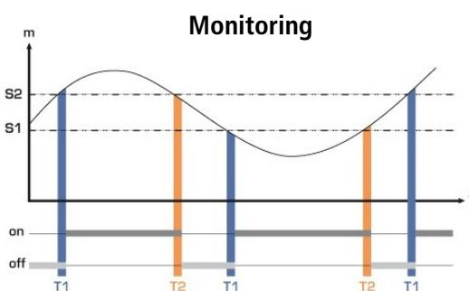
The alarm goes off when the measurement is outside the maximum and minimum threshold.
