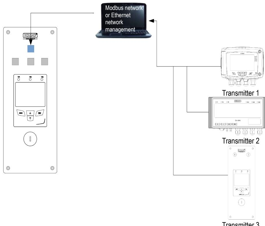
The ATE310 recovers the transmitted data by the transmitters 1, 2 and 3 via the digital input in RS485 or Ethernet and displays them.
