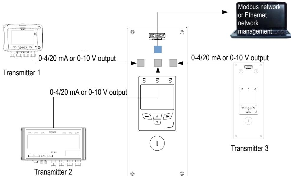
The ATE310 recovers the transmitted data by the transmitters 1, 2 and 3 via the analog inputs and displays them. The ATE310 can also transmit them to a computer via the RS485 or Ethernet connection.
