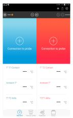
Press "Connection to probe" on the left-hand corner of the screen. The following screen is displayed.
