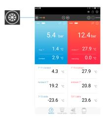
> Press to display the refrigerant gases list.
